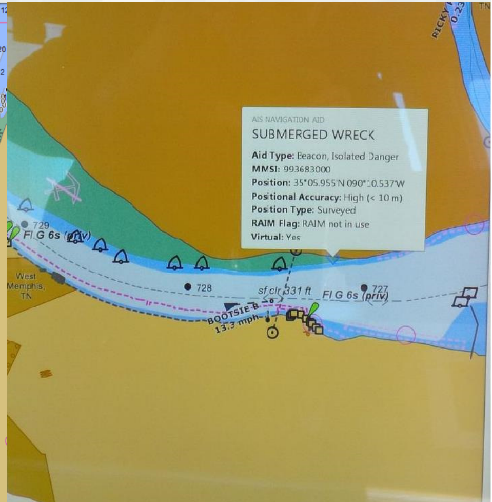
AIS V-AtoN marking submerged wreck in swift river waters
