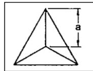
Here is an example: A radar reflector with an inner edge length of 42 cm achieves a reflection area of 128m<sup>2</sup> at a radar frequency of 9.4 GHz ( $\lambda = 3.19$  cm).
