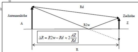
This causes the radar waves from the two spatial directions to overlap. In extreme cases, this multipath propagation can lead to an in-phase addition (+3 dB) or even to complete cancellation if the two waves are in opposite phases. This effect is most pronounced when the sea is calm and decreases as the sea state ("clutter") increases.
