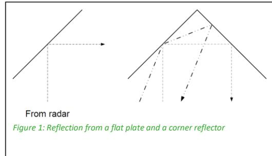
**corner reflector: reflector, consisting of flat conducting surfaces intersecting mutually at right angles, that reflects the greater part of the incident waves parallel to their direction of incidence (ISO 8729)**
