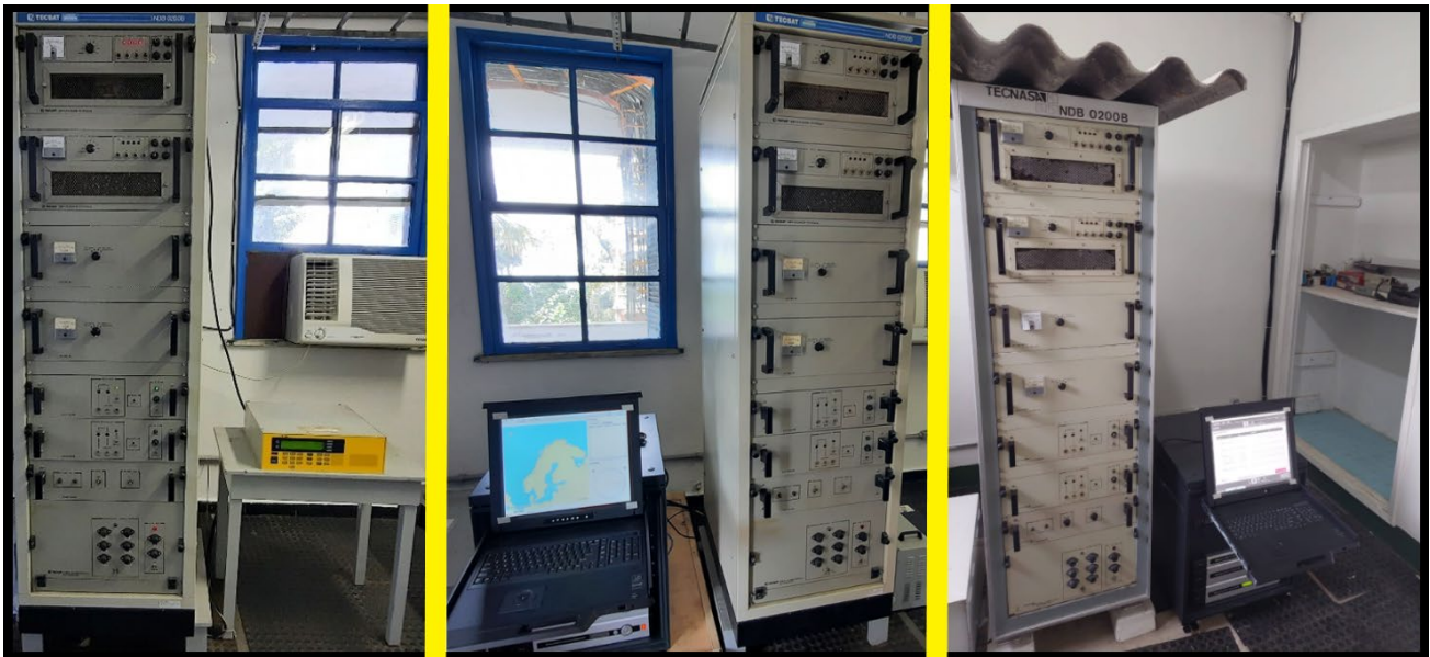
Figure 2: Obsolete Iala Station - Left, Retrofitted Station -Center ( Ilha Rasa Station), Retrofitted Moela Station – Right.
