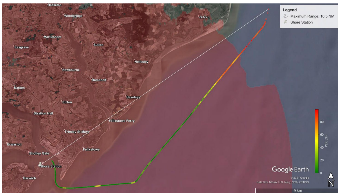
Figure 111: Predicted coverage area in low-power mode (shown in red) and measured Shore-to-ship PER.
