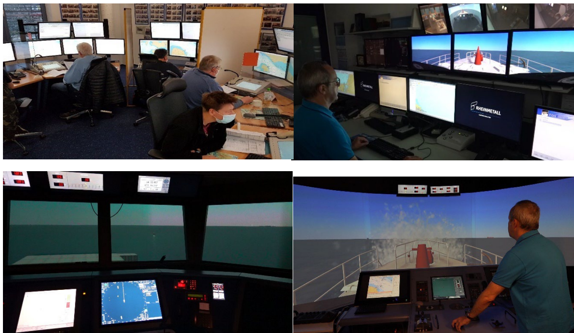
Figure 30: Training exercises in VTS simulator for Fehmarn Belt Tunnel Construction (top left) and scenarios in interfaced Ship Handling (Top right: SHS Instructor station; bottom left: Bridge view from Passing Traffic ship; Bottom right: Bridge view from Guard vessel in action)
