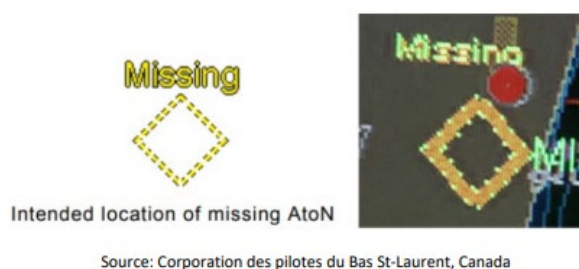
Figure 4 Missing virtual AIS AtoN symbol versus display on ECDIS
