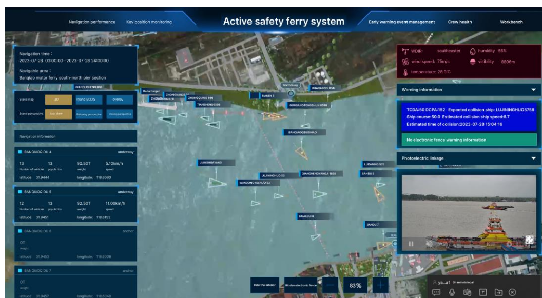
Figure 5: Collision warning system for ferries in ferry waters
