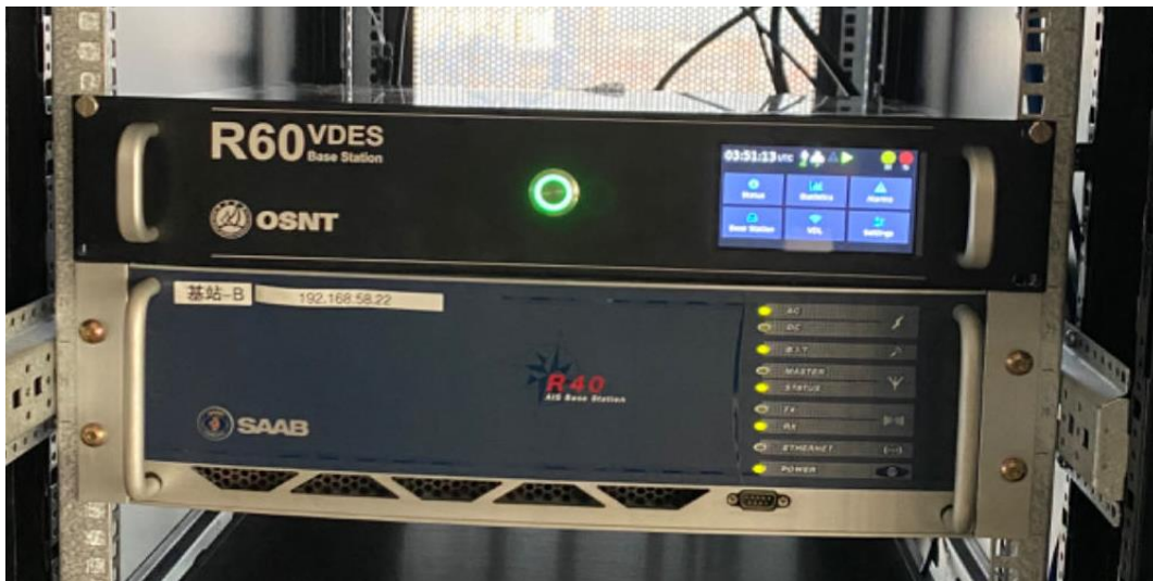
Figure 2 VDES base station installed at the VTS Center
