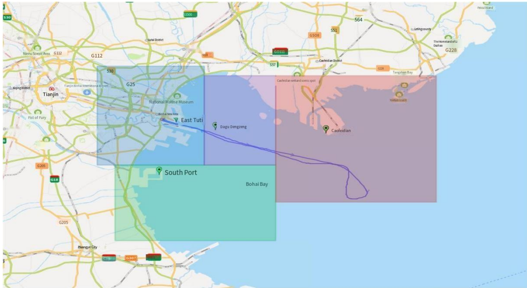
Figure 8 Service area planning of VDES base station in Tianjin Port
