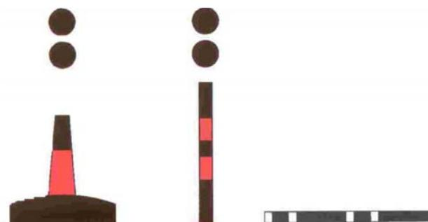
**Note:** <sup>(b)</sup> The double sphere topmark is a very important feature of every Isolated Danger mark by day, and should be used wherever practicable and be as large as possible with a clear separation between the spheres.
