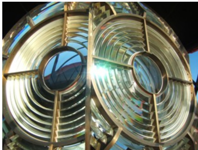
Figure 1 Rotating Multiple Pencil Beam Apparatus at Casquets Lighthouse
