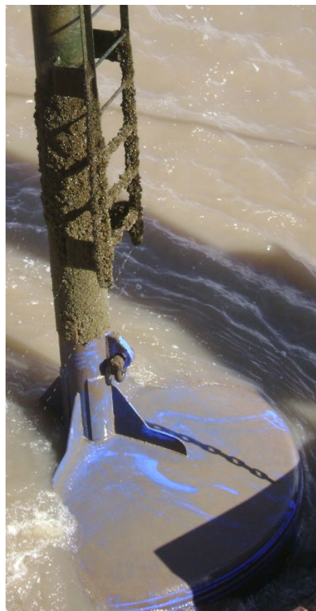
Figure 1 Spar buoy painted with fluoropolymer paint
