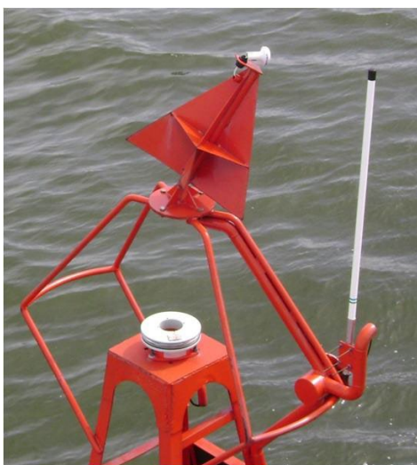
Figure 7 Antenna damage due to collision
