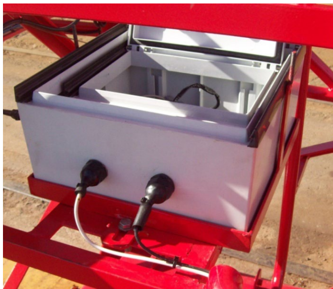
Figure 15 Example of a double enclosure
