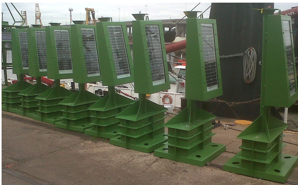
Figure 8 Buoy super-structures with solar panel protected by an impact resistant glass inside a steel box.
