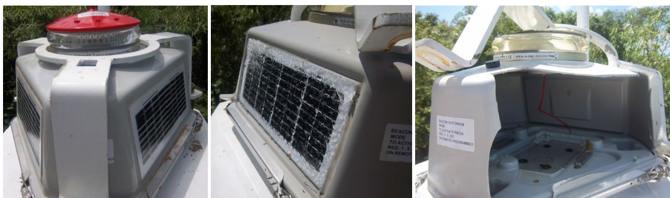
Figure 12 Examples of AtoN where mechanical protection has failed.
