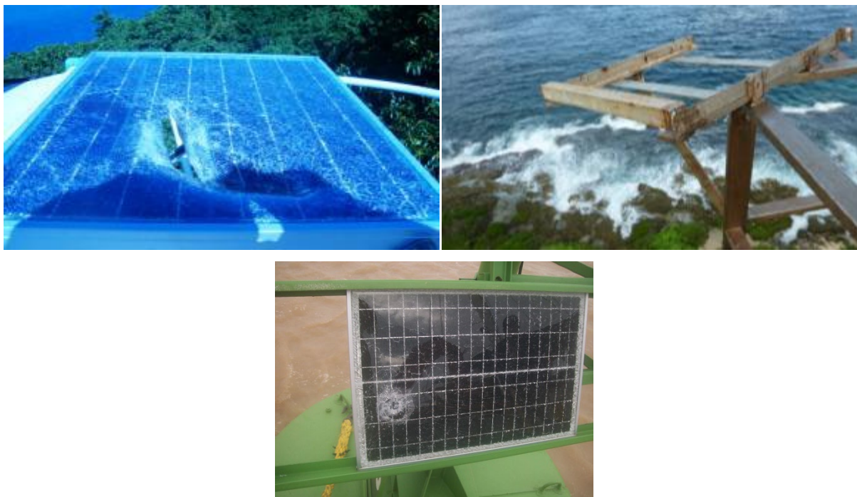
Figure 1 Examples of damage, theft and gunfire to AtoN
