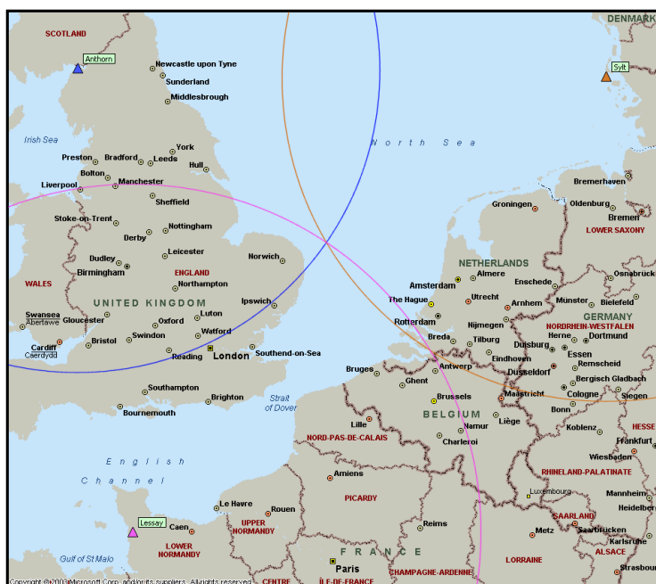
Figure 6 Example of all-in-view positioning using Anthorn, Lessay and Sylt. With all-in-view mode signals need not belong to the same GRI and more than three signals are employed in the positioning solution in order to provide integrity
