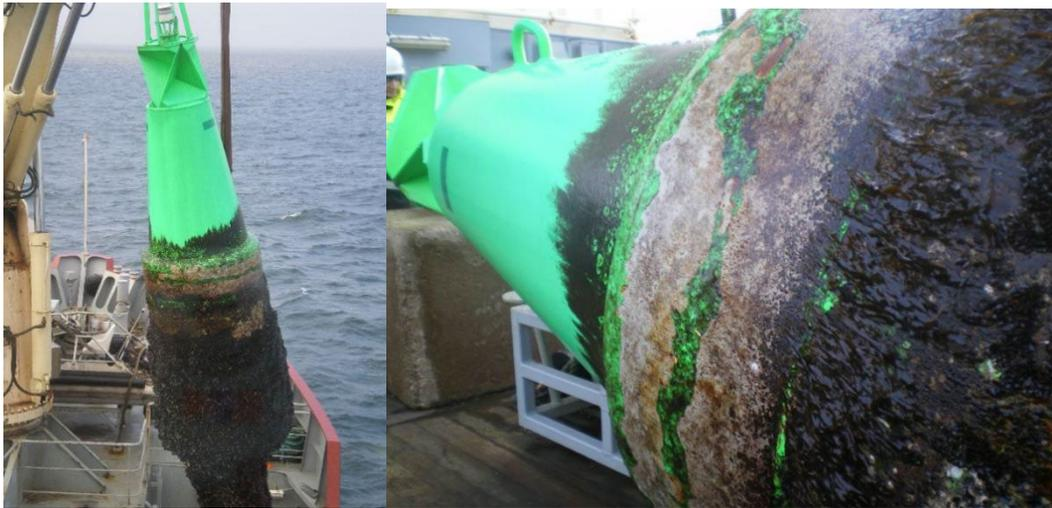
*Figure 4 Coloured part with marine growth should be avoided when evaluating the fading of the colour but included when evaluating the visual day mark colour of the AtoN.*
