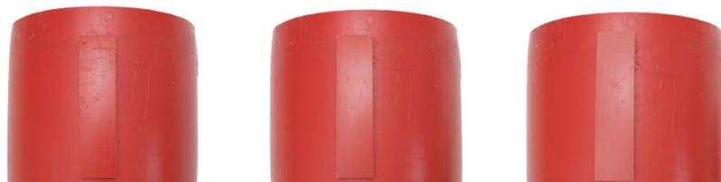
To demonstrate fading, the red colour models have been photographed against new buoy colours in studio conditions.
