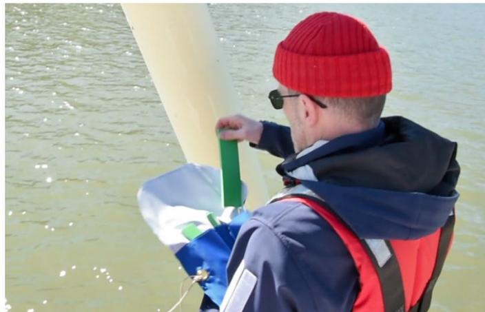
It is easy to assess the fading of navigation buoys with reference samples even in field conditions.
