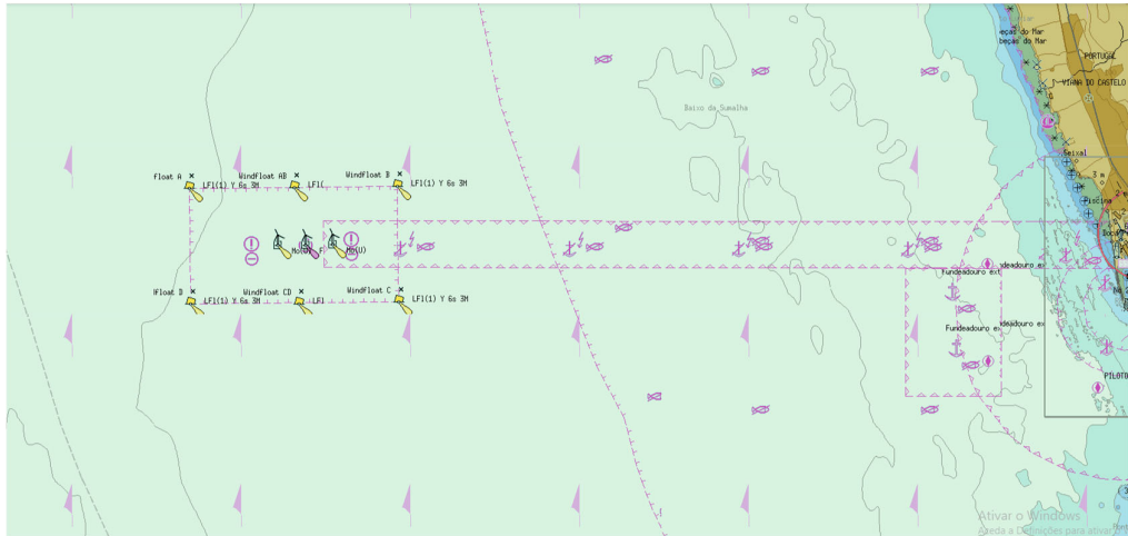
Figure 1 Example of Charted Safety Zone from Portugal
